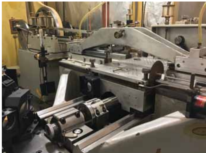
RULING ENGINE “B,” with its much more rigid frame, was a great success. The small mirror mounted to the grating carriage and the optics to the left monitored the line spacing with great precision and made needed corrections as the machine operated.
